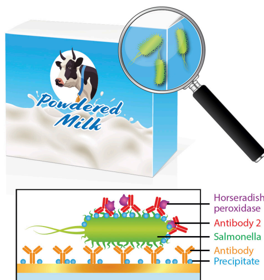
Figure 1. Salmonella detection from powdered milk using Multi-Parametric Surface Plasmon Resonance (MP-SPR). Binding of horseradish peroxidase antibody 2 (HRP-Ab2) specifically on Salmonella and formation of precipitate.
