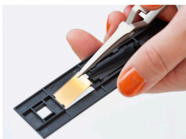
Figure 1. The convenient sensor slide holder of MP-SPR Navi™ allows easy functionalization of a sensor in situ and ex situ . There is a multitude of methods for coating, such as spray coating, CVD, MBE, ALD, sol-gel deposition, Langmuir-Blodgett monolayer depositions, spin coating, dip coating, self-assembly, electrochemistry etc. Additionally, the sensor slide can be further characterized using AFM, SEM or microscopy.
