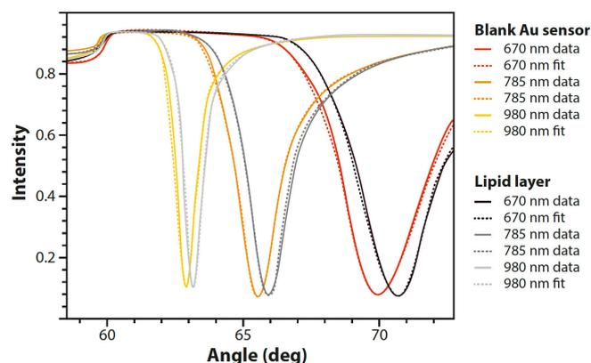
**Figure 3.** MP-SPR curves of supported lipid bilayer (SLB) deposition. The experimental data was fitted using LayerSolver™ software.
