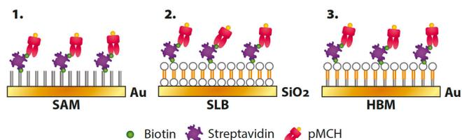
**Figure 1.** Different sensor formats: 1. Au coated with PEGylated SAM. 2. SiO<sub>2</sub> with SLB. 3. Au coated with HBM. All 3 surfaces were modified with biotin moieties, streptavidin and pMHC.
