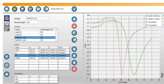
Figure 5. MP-SPR Navi™ LayerSolver™ can be used to fit measured SPR curves to determine thickness and RI of the deposited layer.
